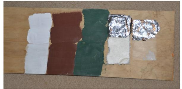
**Three coloured paint areas, additive added to the top areas. Insulation plus foil then just insulation on right**
