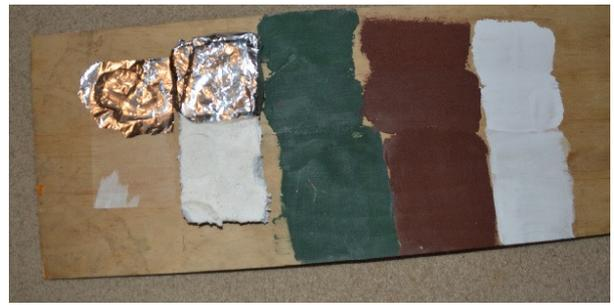
**Foil on the left, then insulation plus foil and insulation. Three coloured paint areas on the right, additive added to the top areas**
