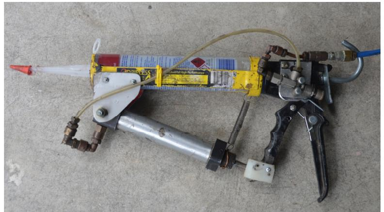
*A silicon gun operate by an air compressor*
